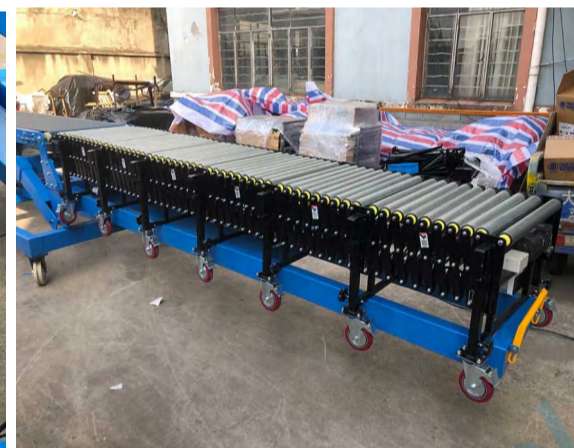
7.2m flexible powered roller conveyor
