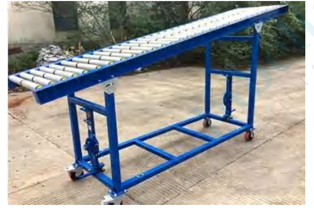
The declined section is height adjustable
