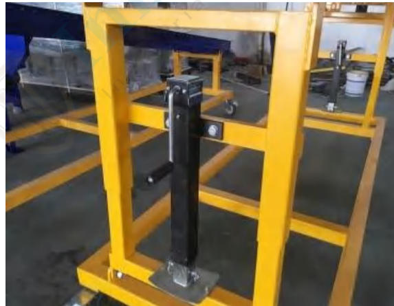
Screw jack and adjustable height on each deck
