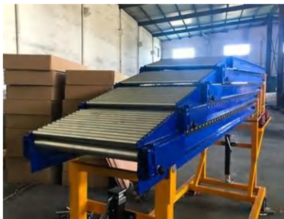
25mm diameter steel rollers within a transfer slider section.
